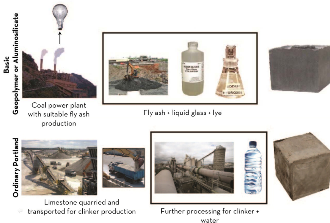
Figure 19. Manufacturing Differences Between 'Geopolymer' and Portland Cement [53,49]
